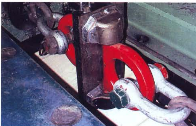
Production control at RUD. Breaking test of a RUD RBS 50t lifting point with a minimum breaking strength of 2000 kN.
